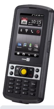
Rugged Smartphone with Windows Mobile (PDA), built-in barcode reader, camera and GPS. Unlike similar products, this one has widescreen WQVGA screen and the control environment SPB Shell 3D.
